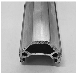
Figure 8 The profile obtained by mold testing
