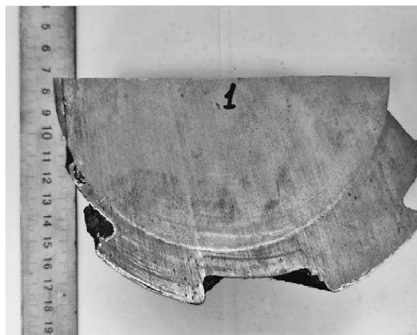
Figure 2 Example of a steel nipple with cast-iron casting
