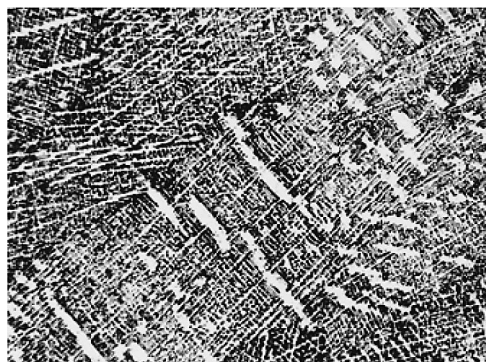
Figure 4 The microstructure of the casting after blowing B10 scrap with compressed air, magnification of 100 x
