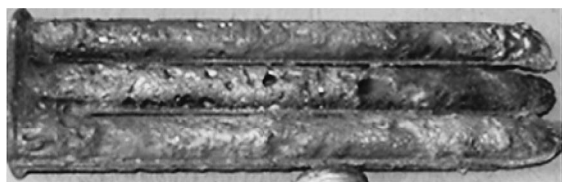
Figure 1 A casting made of melted ingots of B10 alloy
