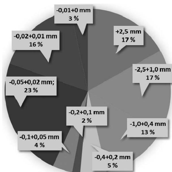
Figure 1 Granulometric characteristics of kaolin raw materials
