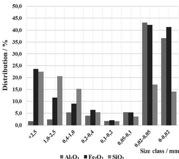
Figure 2 Distribution of major elements by size classes in kaolin raw material
