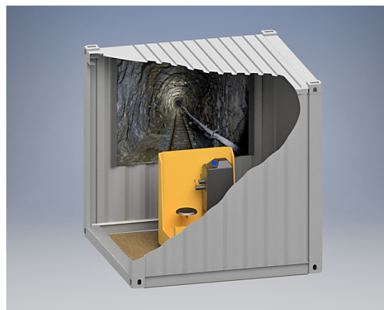
Figure 7: Displaying a 3D panorama of a real mine with one projection screen
