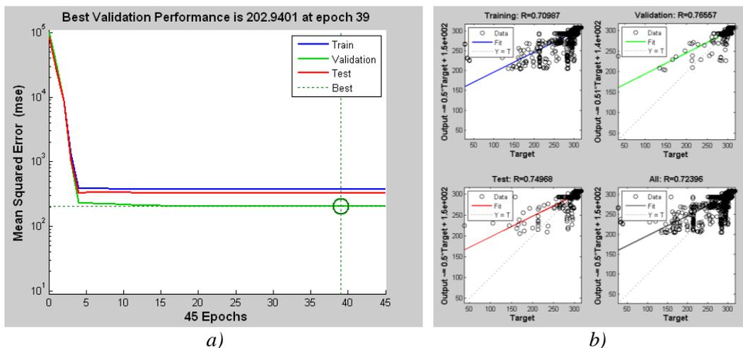
Figure 4. The efficiency of multi-layer feed-forward neural network determined by: a) mean squared error, b) regression plot.
