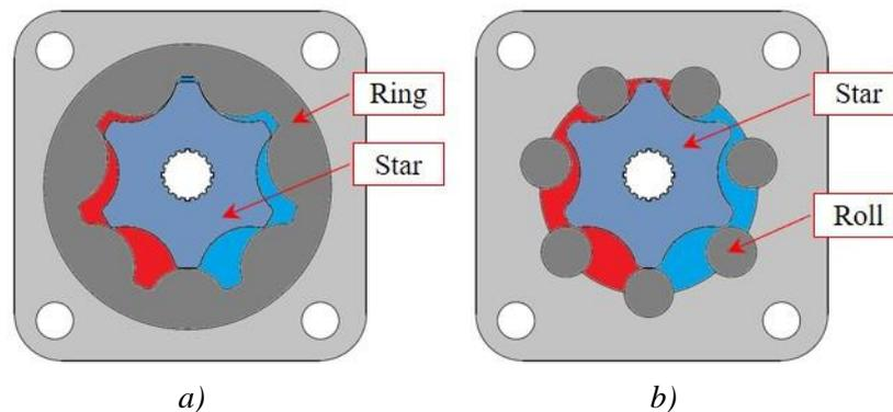
Figure 1. Working principle of: a) GEROTOR motor, b) GEROLER motor
