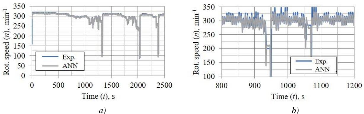
Figure 8. Results of the hydraulic motor rotational speed by the NARX dynamic neural network: a) for learning measurement data b) for new measurement data.
