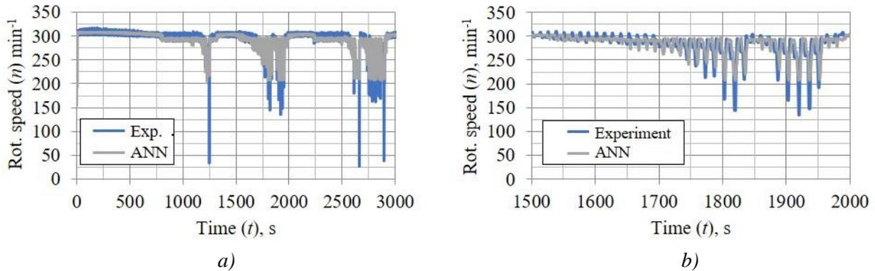
Figure 6. Results of the hydraulic motor rotational speed by the multi-layer feed-forward neural network for learning measurement data.
