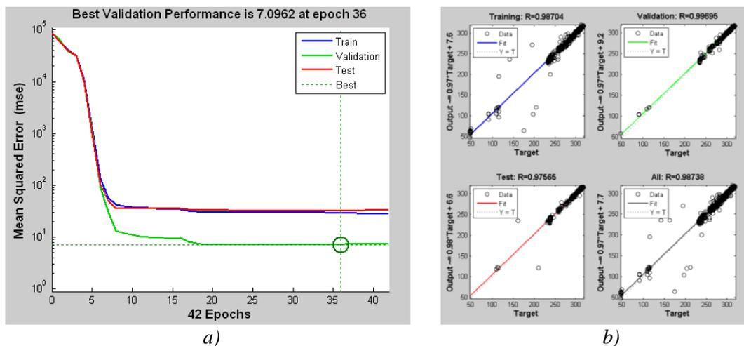
Figure 5. The efficiency of the NARX dynamic neural network defined by: a) mean squared error, b) regression plot.
