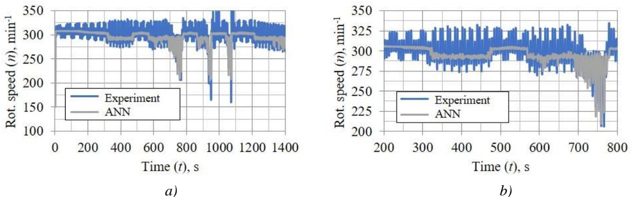
Figure 7. Results of the hydraulic motor rotational speed by the multi-layer feed-forward neural network for new measurement data
