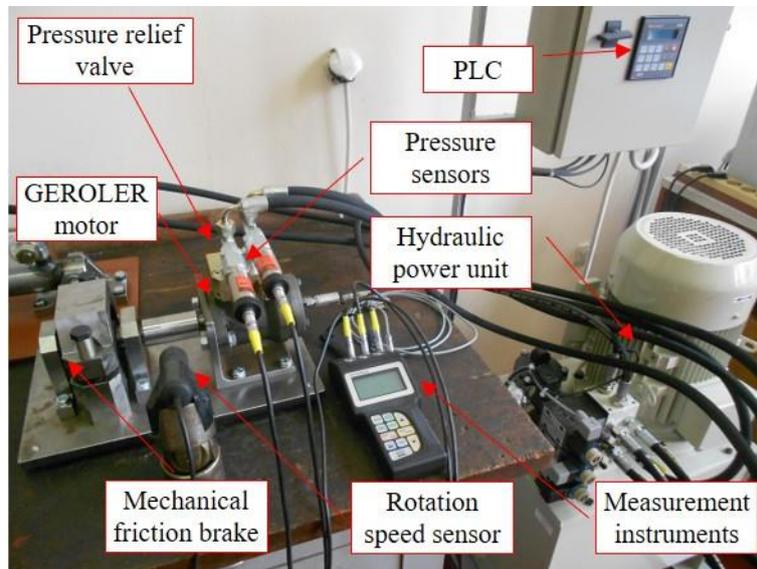
Figure 2. Laboratory hydraulic system for measuring the GEROLER motor operating parameters.
