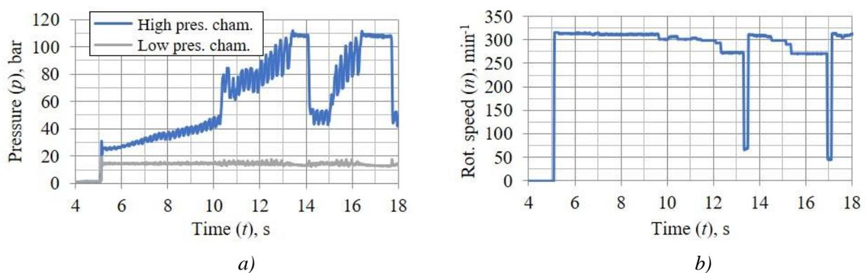
Figure 3. Measurement results of the hydraulic motor: a) pressure in the high- and low-pressure chamber, b) rotational speed.
