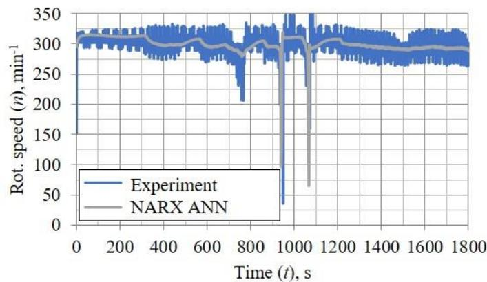
Figure 9. Results of the hydraulic motor rotational speed by the NARX dynamic neural network with the closed loop parallel form.
