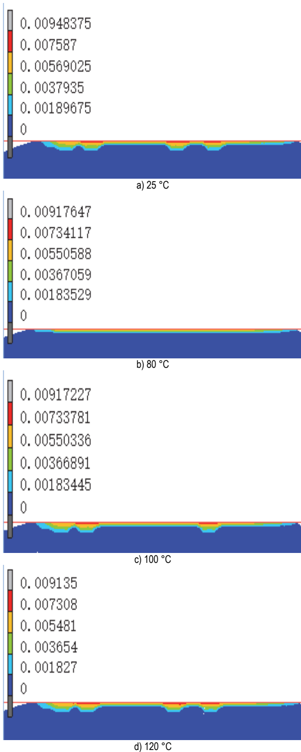
Figure 18 Cloud chart of cumulative wear rate
