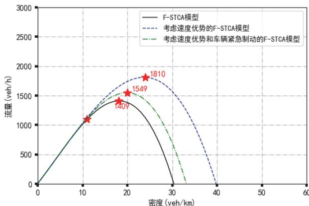
Figure 12 Road capacity analysis under different models
