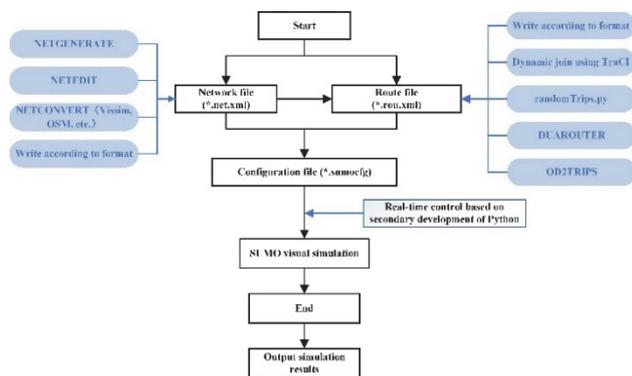
Figure 6 Simulation flow chart of SUMO
