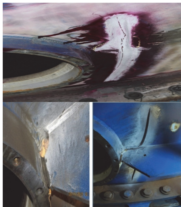
Figure 1 Crack samples on the discharge ring
