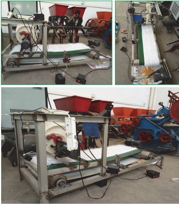
Figure 4 Structure of cell-wheel precision seed-metering device
