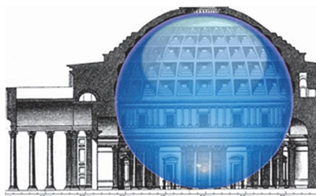
Figure 4 Pantheon cross-section with 43.3-metre diameter sphere fitting under its dome, [10]
