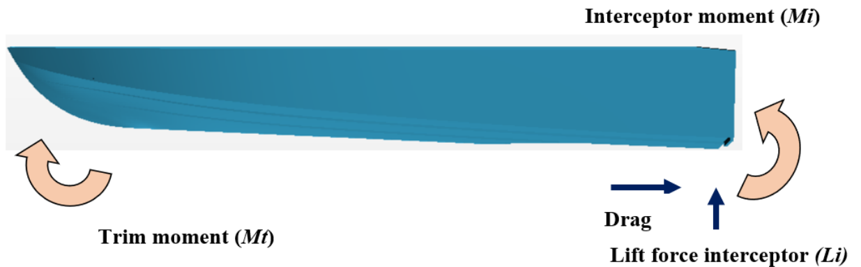
Fig. 11 Moments and forces generated by the interceptor
