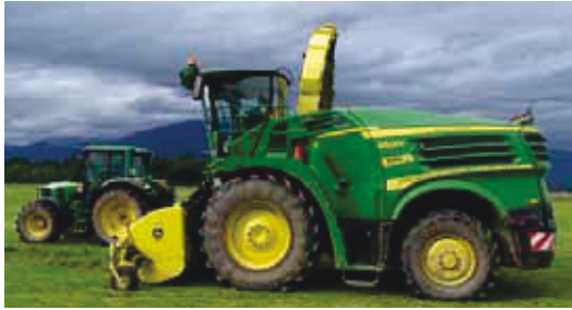
Slika 1. Samokretni silažni kombajn John Deere 8500i Figure 1 The John Deere 8500i self-propelled forage harvester
