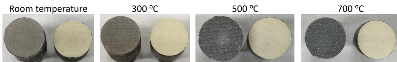
**Figure 3.** Fractured surface of substrate and TiO<sub>2</sub> coating after tensile strength test
