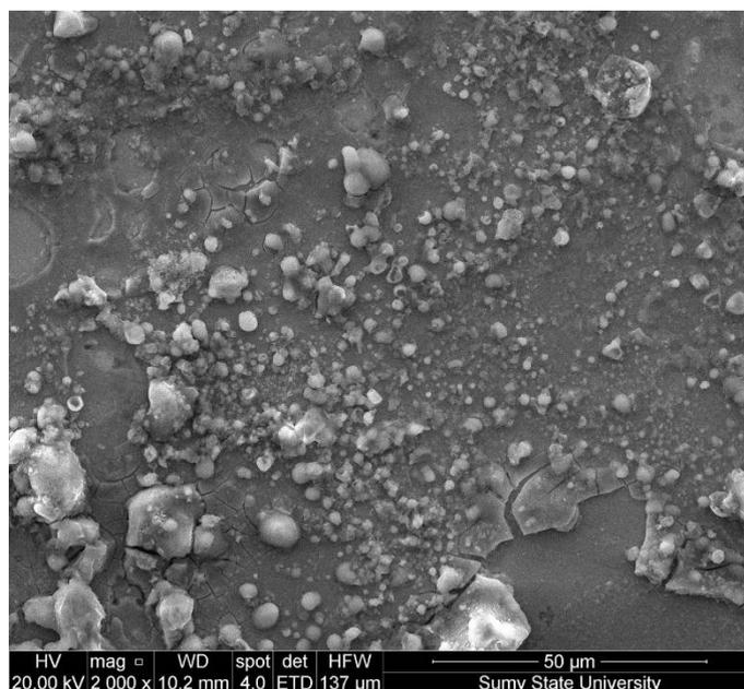
**Figure 3.** SEM image of por-InP surface with the nickel-containing surface layer
