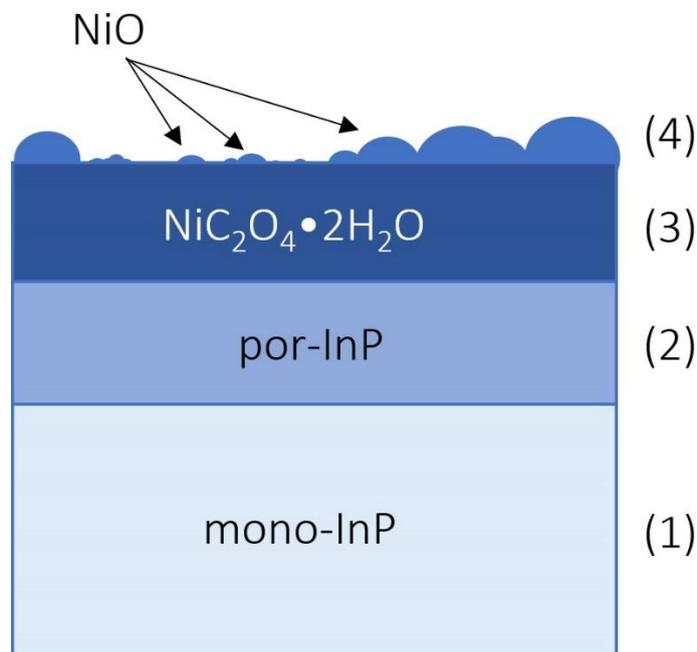
**Figure 6.** Schematic image of NiO/NiC<sub>2</sub>O<sub>4</sub>·2H<sub>2</sub>O/por-InP/mono-InP structure
