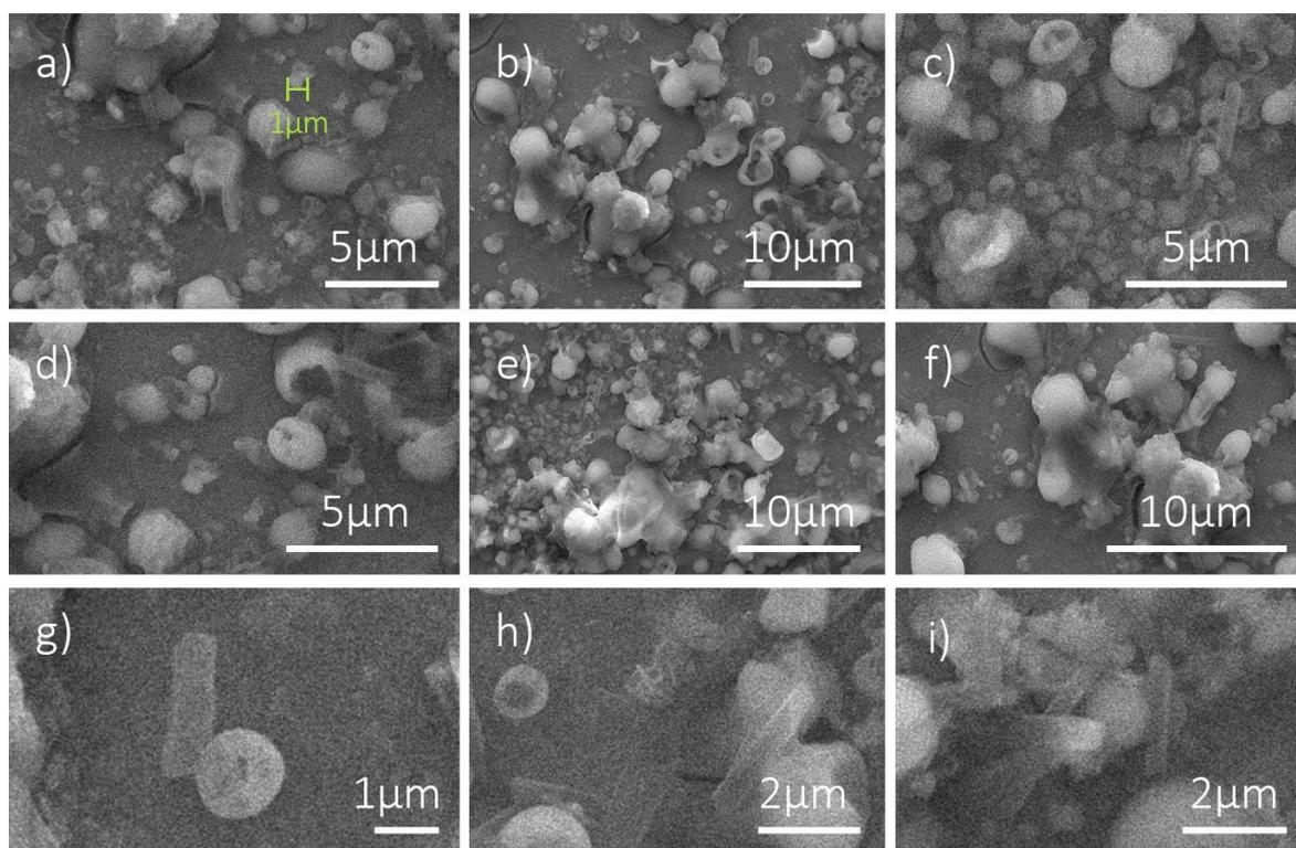
**Figure 5.** SEM images of NiO crystallites and nanocrystallites
