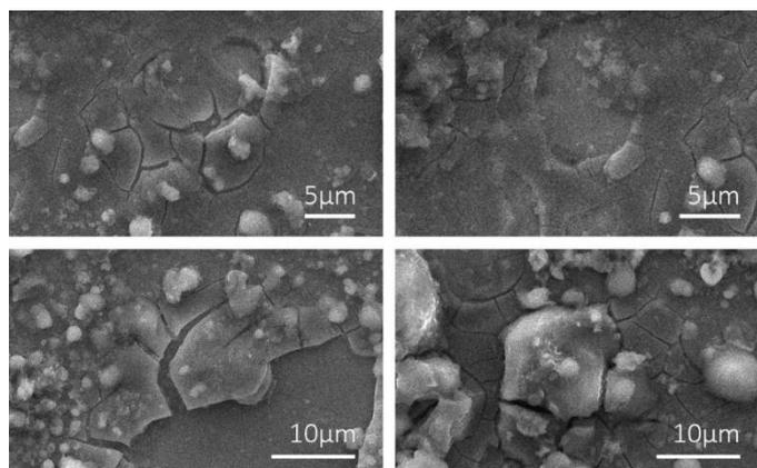
**Figure 7.** SEM images of NiO/NiC<sub>2</sub>O<sub>4</sub>·2H<sub>2</sub>O/por-InP/mono-InP structure surface
