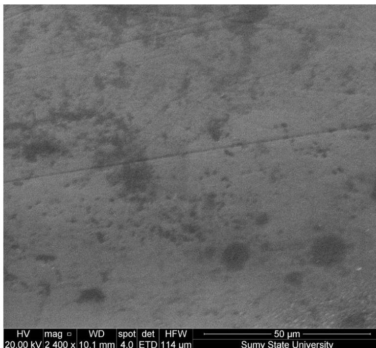
**Figure 1.** SEM image of the morphology of por-InP porous surface
