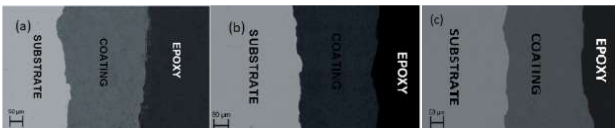
Figure 4. Cross-sectional morphology of HVOF sprayed coatings: (a) Cr 3 C 2 -25NiCr; (b) 5 wt.% YSZ- (Cr 3 C 2 -25NiCr); (c) 10 wt.% YSZ- (Cr 3 C 2 -25NiCr)
