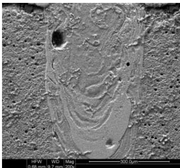
Figure 6. SEM image of laser modified HVOF thermally sprayed Inconel 625 and WC-12Co coatings; laser power 170 W. laser scan speed 1750 mm min -1 . micro structured powder
