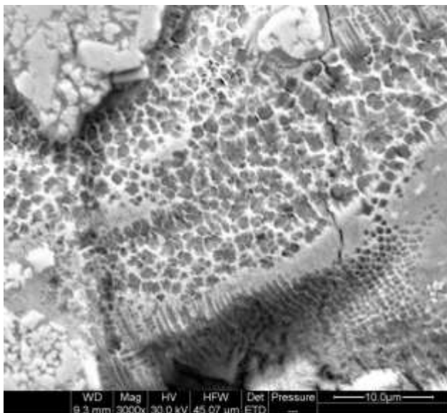
Figure 3. SEM image of laser modified HVOF thermally sprayed Inconel 625 and WC-12Co coatings; laser power 55 W laser scan speed = 1250 mm min -1 nanostructured powder
