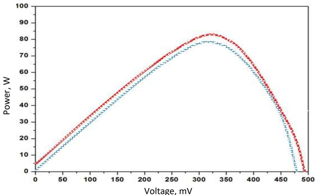
**Figure 10.** P-V characterization of (—)TO and (—) CTO thin film on GCE in 0.1 M KCl (dye coated substrate)
