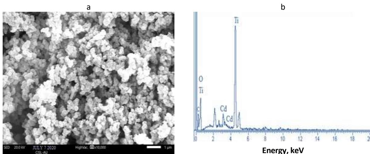
**Figure 1.** (a) SEM image and (b) EDS analysis of Cd  $\text{TiO}_2$  (CTO) film
