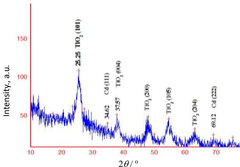
Figure 3. XRD analysis of CTO thin film
