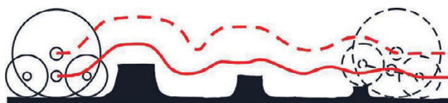
Slika 2. Usporedba kretanja bogi i jednostruke osovine Fig. 2 Comparison of axle movement on bogie and single axle
