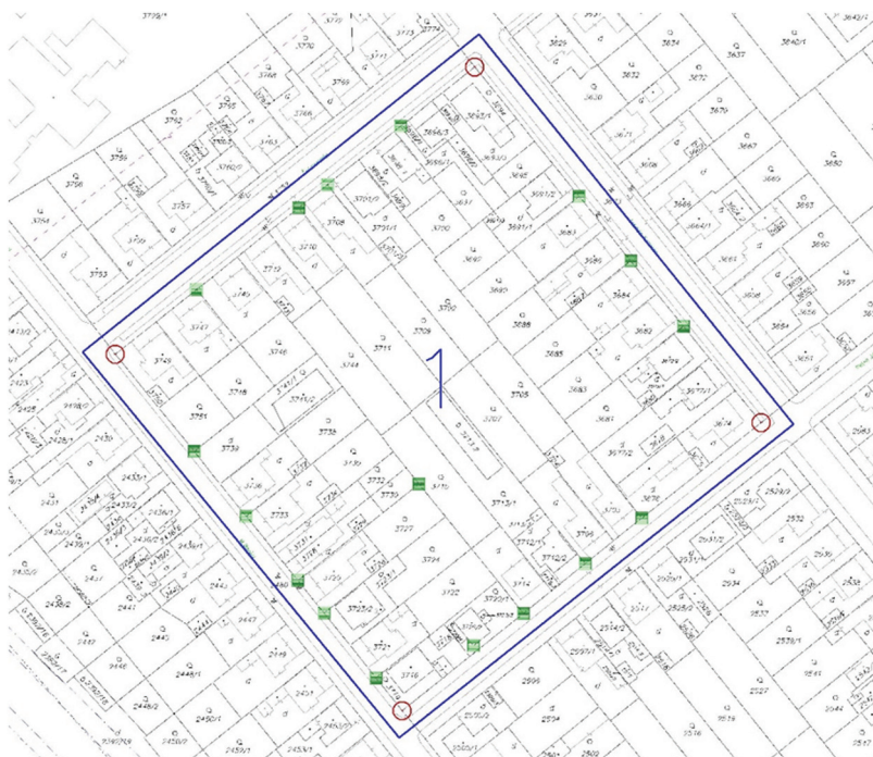
Fig. 5. Ideal configuration of identical points (red circle) and check points (green square).
