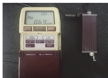
Figure 2 Mitutoyo SJ-201 brand surface roughness measuring device
