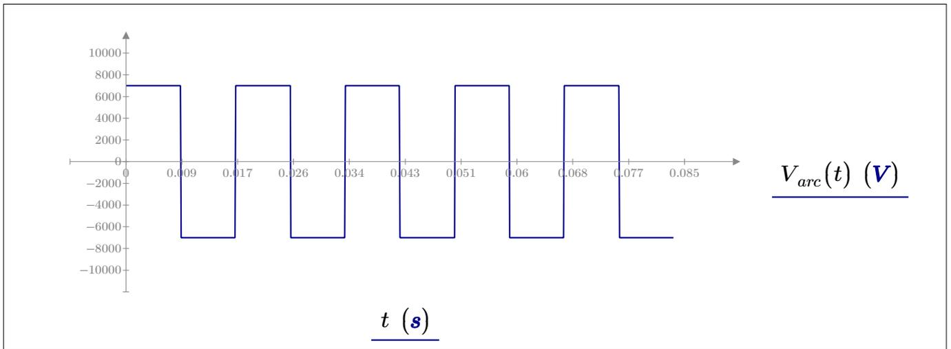
Figure 4. Typical waveform of arc voltage
