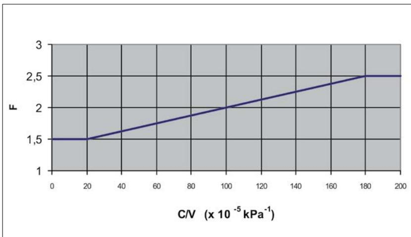
Figure 5. Variation of the dynamic amplification factor F for Equation (2)
