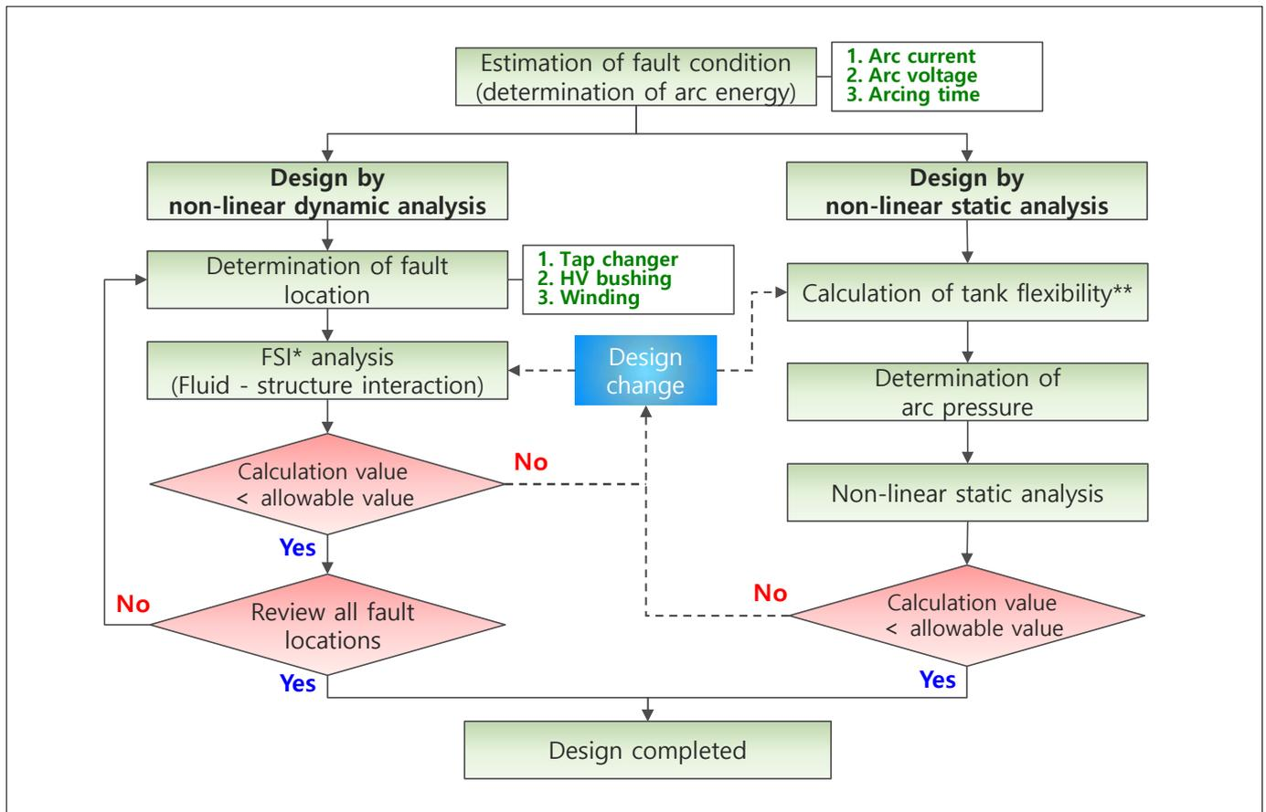
Figure 2. Tank design process
