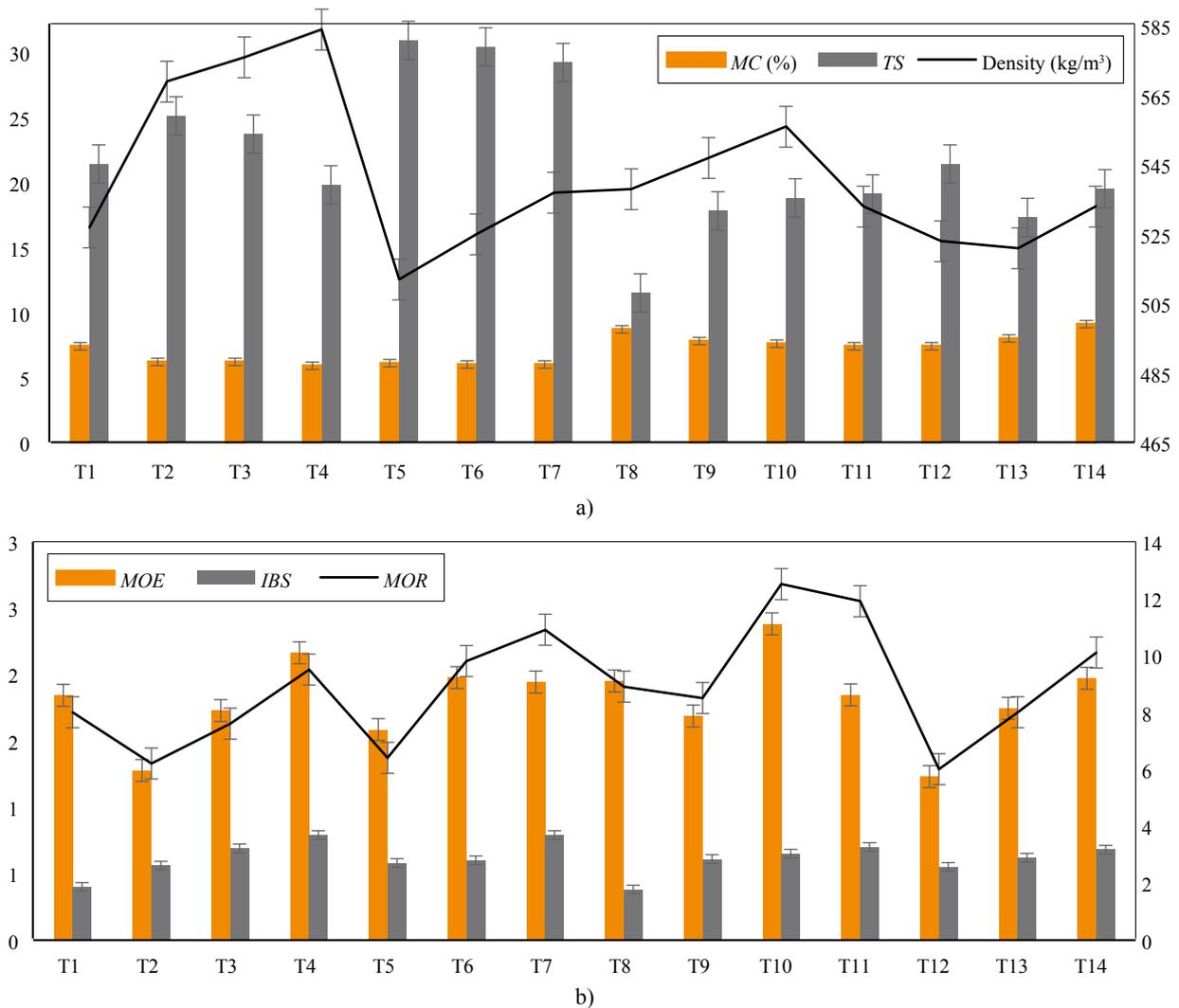
**Figure 3** a) Physical and b) mechanical properties of particleboards
