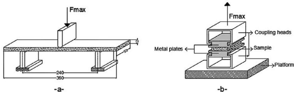
**Figure 4** Test configuration: (a) bending strength, (b) internal bond strength
