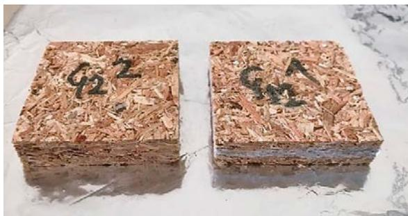
**Figure 5** Internal bond strength test samples
