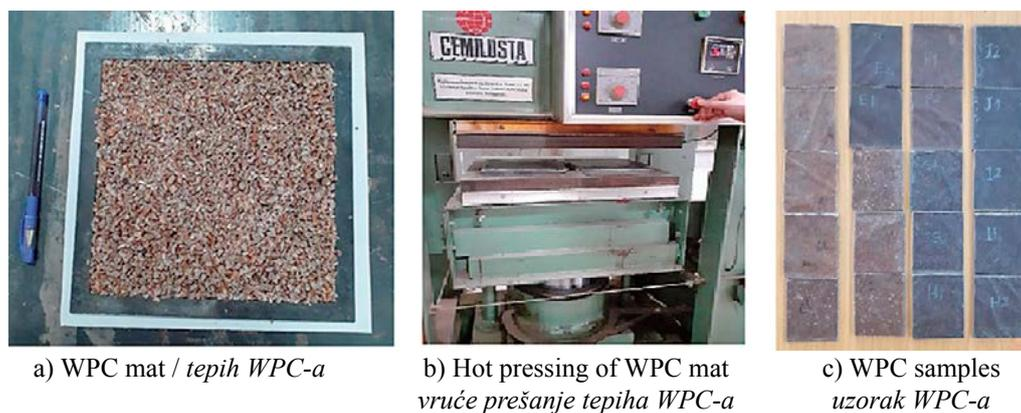
**Figure 2** Hot-press molding of WPC granules and resulting WPC specimens
