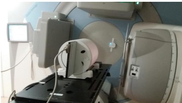
Figure 1. PTW Octavius 4D dosimetric system set up for measurement at linac couch.
