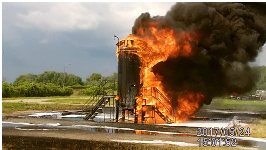
Figure 13. Fire test of a pressure vessel (own photo).
