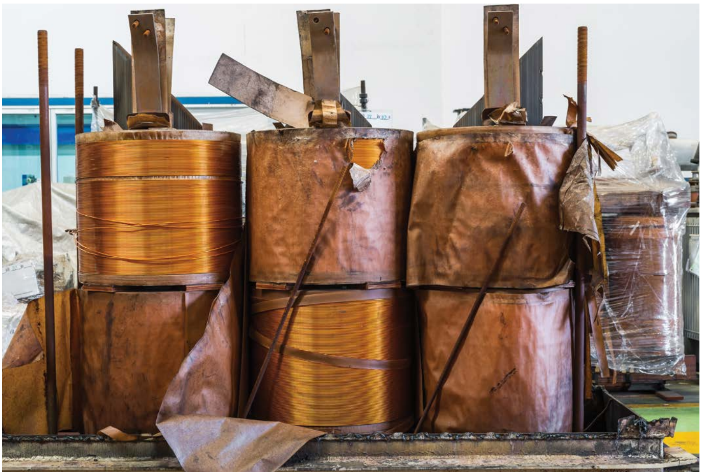
Figure 3. Post-mortem inspection - the compulsory stage for successful transformer health assessment and for AI
