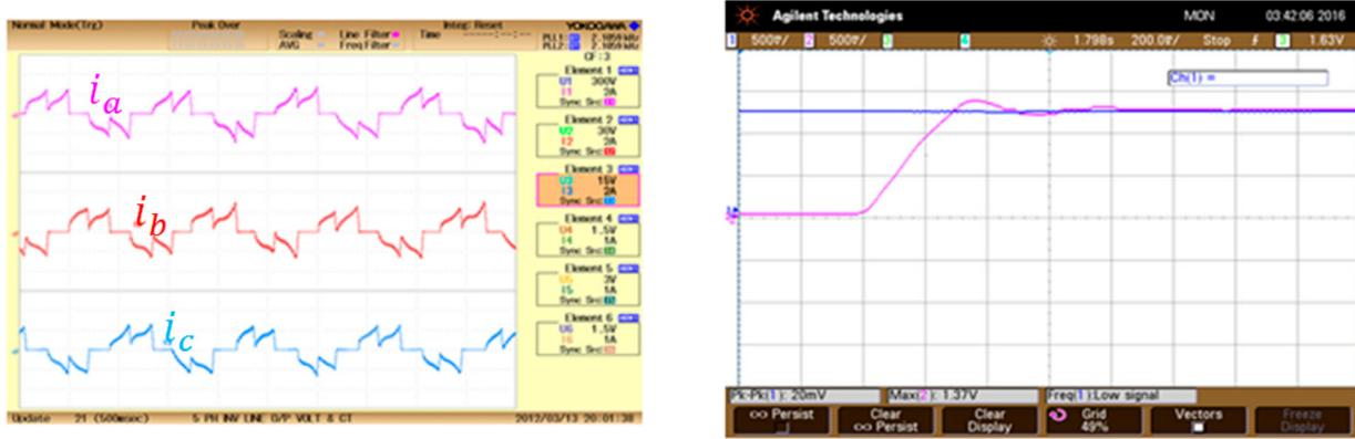
Figure 18. (a) Current waveform of BLDC motor and (b) speed waveform of BLDC motor.
