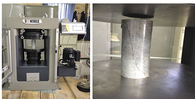
Figure 3: Determination of uniaxial compressive strength (UCS) of studied rock types
