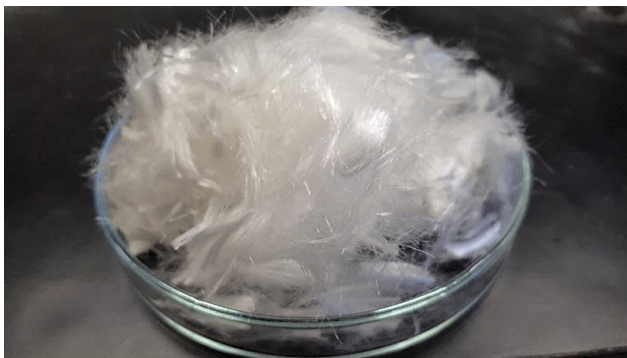
Figure 4: PPFs structure manufactured by the EAMIC company
