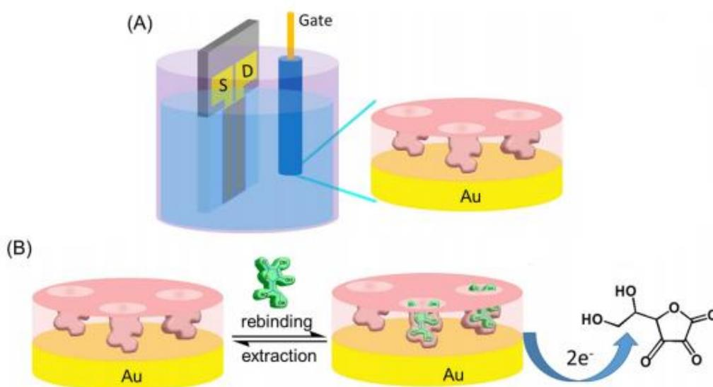
**Figure 5.** (A) Schematic process of MIP-modified OECT sensor for AA detection. (B) Schematic process of AA removing and rebinding on surface of MIP film and of AA oxidation on surface of modified gate electrode [173]
