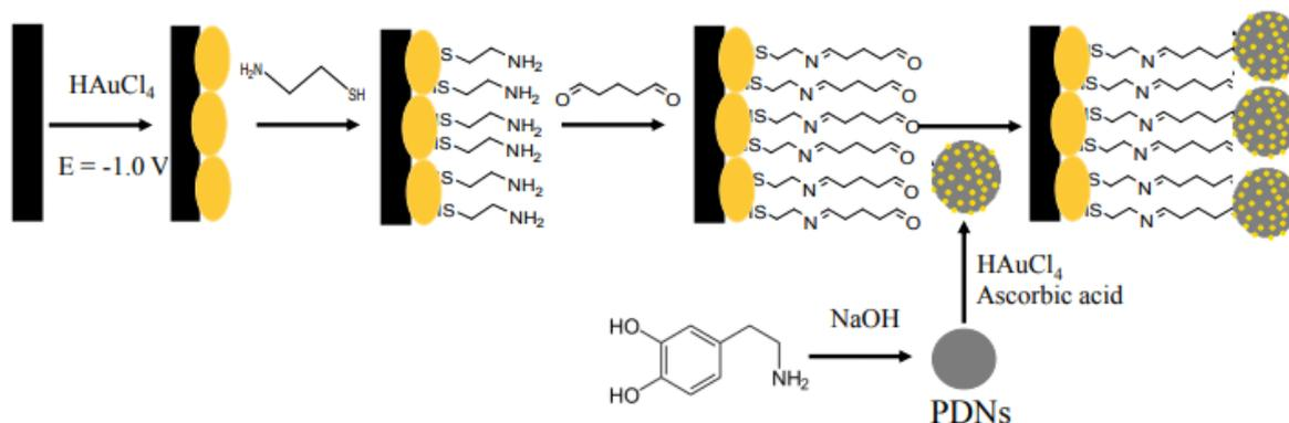
**Figure 1.** Schematic process of electrode preparation [158]
