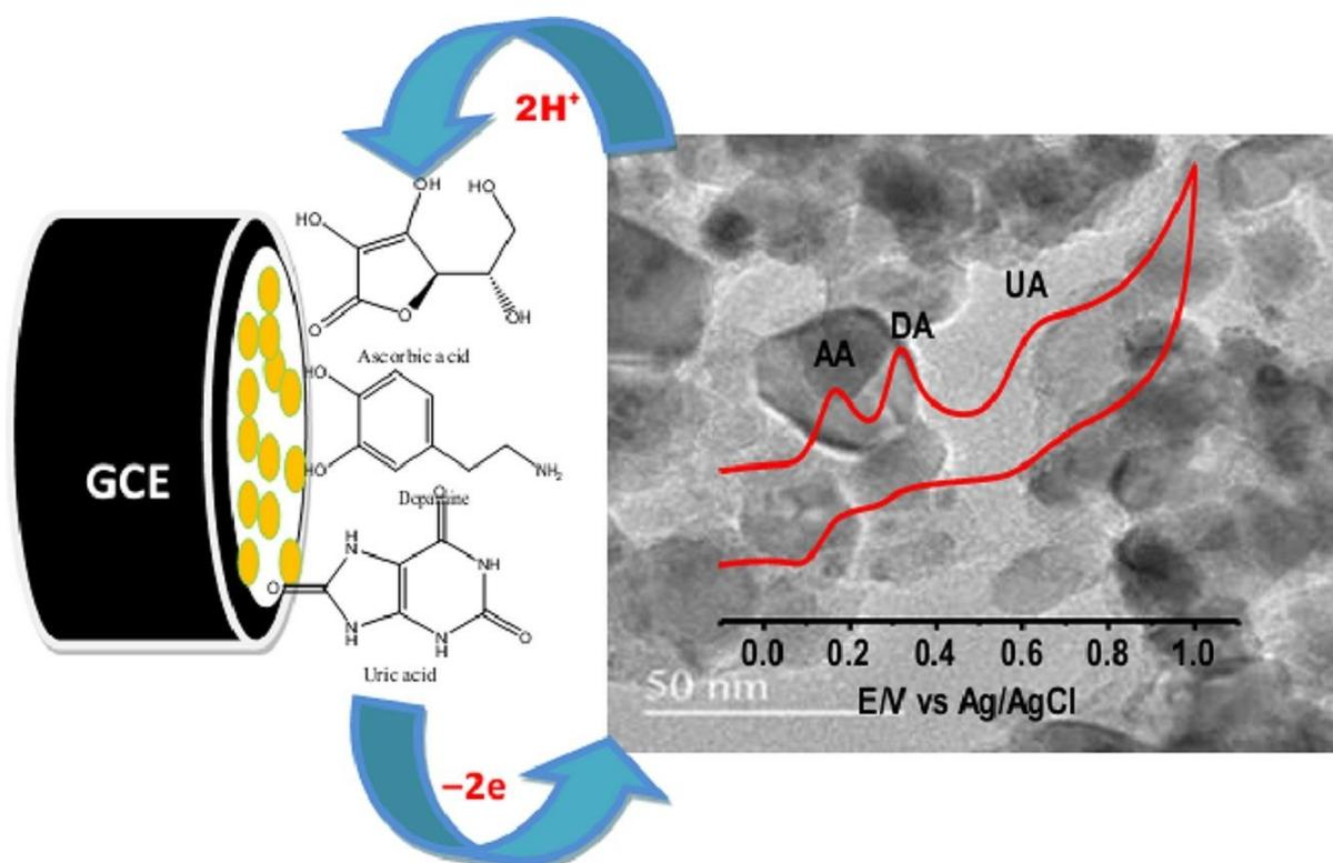
**Figure 2.** Schematic process of glassy carbon electrode modified with  $\text{SnO}_2$ /chitosan (CHIT) nanocomposite to co-detect AA, DA and UA [161]
