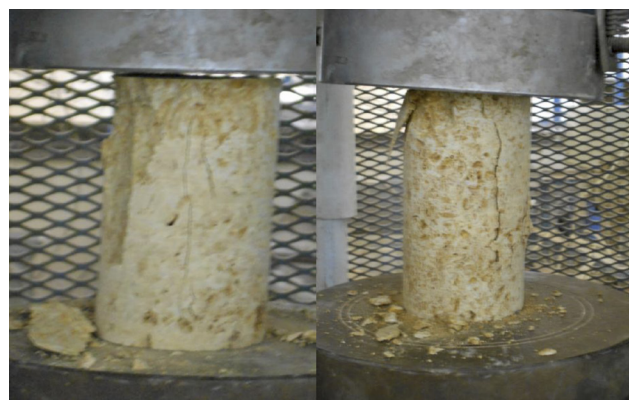
Figure 3: Photos of failure for a limestone sample using a Universal Machine
