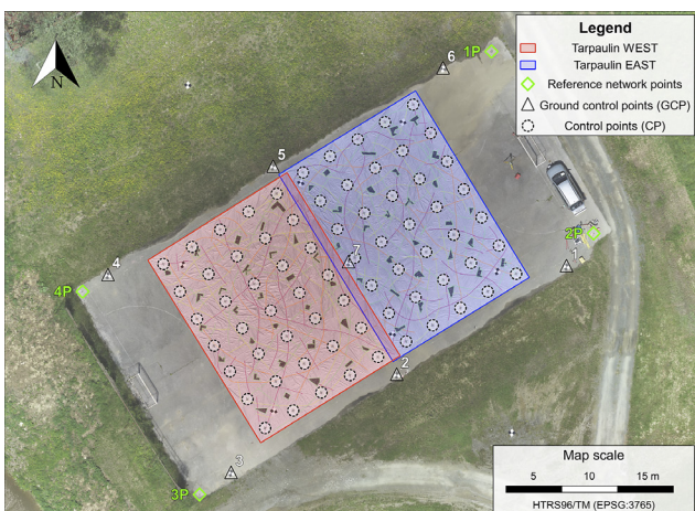
Figure 4: Distribution of the reference network points, CPs, and GCPs on tarpaulins
