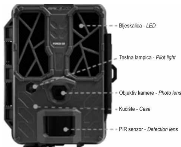
Slika 1. Fotozamka SpyPoint Force-20 s osnovnim dijelovima (Izvor: https://www.manualslib.com/manual/1594013/Spypoint-Force-20.html?page=3#manual )
