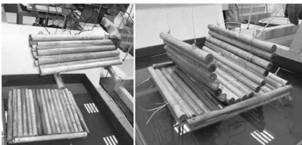
Fig. 5 Lifting of the first row of a flat raft: on left – NArFU construction; on right – VSUT construction
