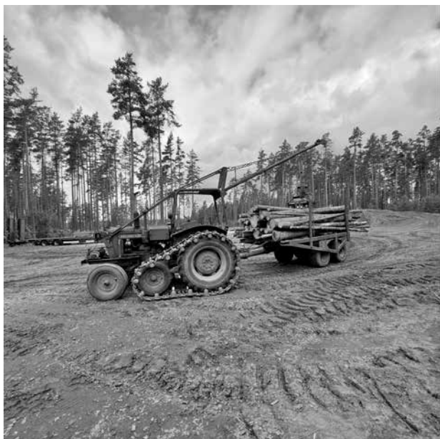
Slika 6. Trakotska ekipaža s mehaničkim kranom i vitlom Fig. 6 Tractor assembly with mechanical crane and winch
