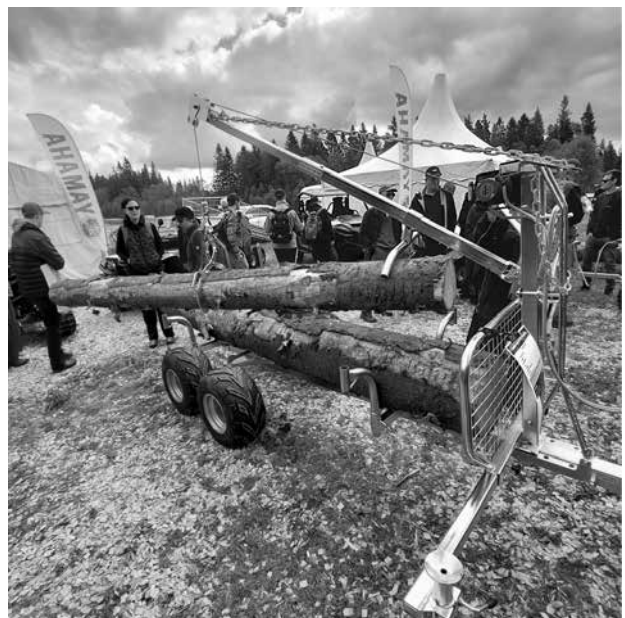
Slika 2. Poluprikolica s mehaničkim kranom i vitlom za ATV Fig. 2 A semi-trailer with mechanical crane and winch for atv
