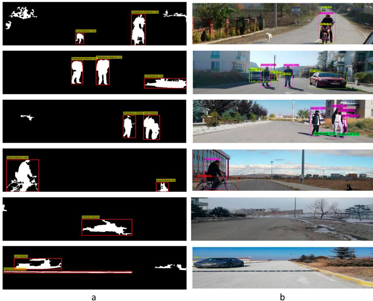
**Figure 11.** Recognized objects using (a) ICANN, (b) YOLO v3.
