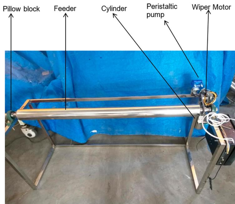
Figure 5. Feeder module.
