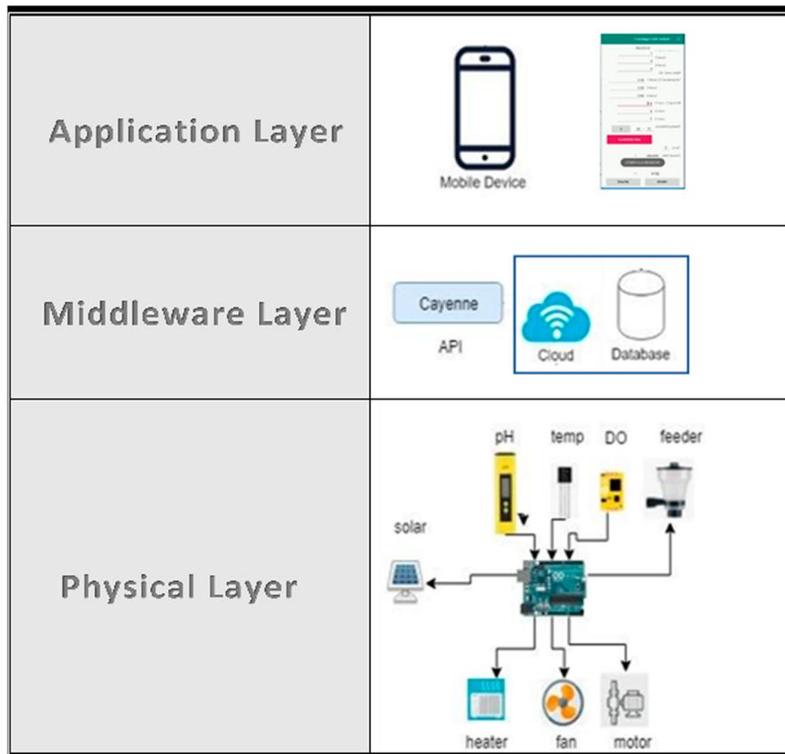
**Figure 1.** Three-layer architecture [17].
