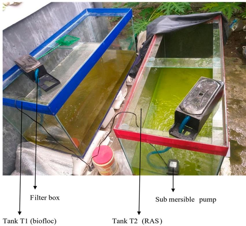
Figure 11. Experimental setup.
