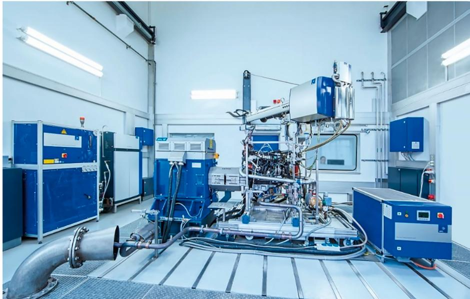
**Figure 8.** The engine test bench can be used to simulate how the rest of the vehicle interacts with a real engine.
