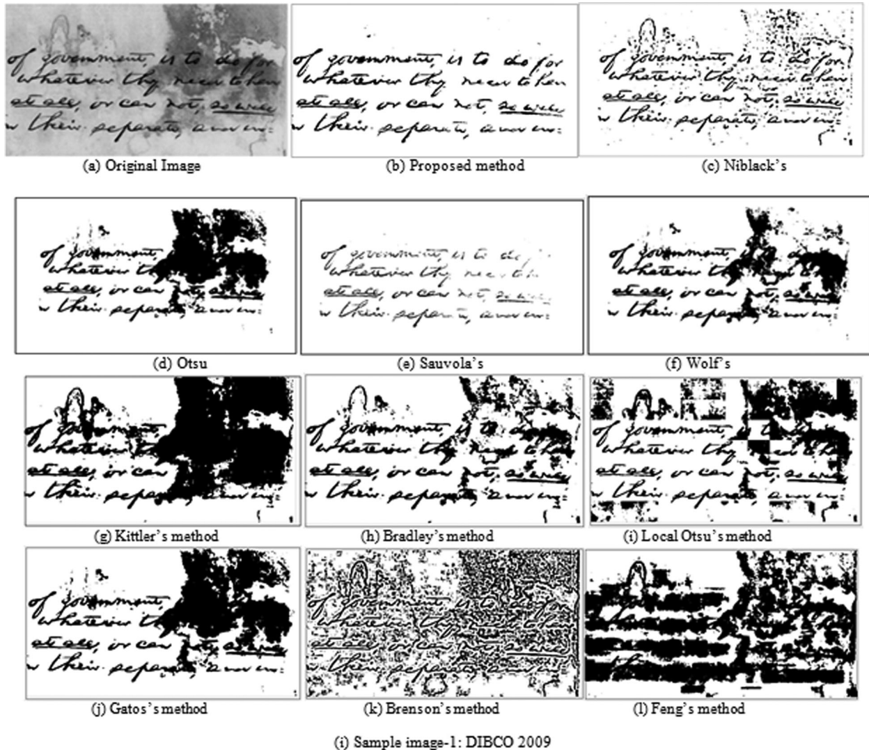
Figure 12. Outcome of proposed method versus state of art methods. (i). Sample image-1: DIBCO 2009, (a) Original Image, (b) Proposed method, (c) Niblack's, (d) Otsu, (e) Sauvola's, (f) Wolf's, (g) Kittler's method, (h) Bradley's method, (i) Local Otsu's method, (j) Gatos's method, (k) Brenson's method, (l) Feng's method. (ii). Sample image-2: DIBCO 2013, (a) Original image, (b) Proposed method, (c) Niblack's, (d) Otsu, (e) Sauvola's, (f) Wolf's, (g) Kittler's method, (h) Bradley's method, (i) Local Otsu's, (j) Gato's method, (k) Brenson's method, (l) Feng's method. (iii). Sample image-3: DIBCO 2017, (a) Original image, (b) Proposed method, (c) Niblack's, (d) Otsu, (e) Sauvola's, (f) Wolf's, (g) Kittler's method, (h) Bradley's method, (i) Local Otsu's, (j) Gato's method, (k) Brenson's method, (l) Feng's method. (iv). Sample image-4: DIBCO 2018, (a) Original image, (b) Proposed method, (c) Niblack's, (d) Otsu, (e) Sauvola's, (f) Wolf's, (g) Kittler's method, (h) Bradley's method, (i) Local Otsu's, (j) Gato's method, (k) Brenson's method, (l) Feng's method. (v). Sample image-5: DIBCO 2011, (a) Original image, (b) Proposed method, (c) Niblack's, (d) Otsu's, (e) Sauvola's, (f) Wolf's, (g) Kittler's method, (h) Bradley's method, (i) Local Otsu's, (j) Gato's method, (k) Brenson's method, (l) Feng's method. (vi). Palm leaf sample image-1, (a) Original image, (b) Proposed method, (c) Niblack's, (d) Otsu's, (e) Sauvola's, (f) Wolf's, (g) Kittler's method, (h) Bradley's method, (i) Local Otsu's, (j) Gato's method, (k) Brenson's method, (l) Feng's method. (vii). Palm leaf sample image-2, (a) Original image, (b) Proposed method, (c) Niblack's, (d) Otsu's, (e) Sauvola's, (f) Wolf's, (g) Kittler's method, (h) Bradley's method, (i) Local Otsu's, (j) Gato's method, (k) Brenson's method, (l) Feng's method.
