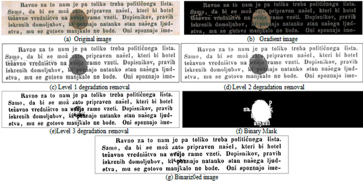
Figure 10. Proposed binarization algorithm – results presented. (a) Original image, (b) Gradient image, (c) Level 1 degradation removal, (d) Level 2 degradation removal, (e) Level 3 degradation removal, (f) Binary Mask, (g) Binarized image.
