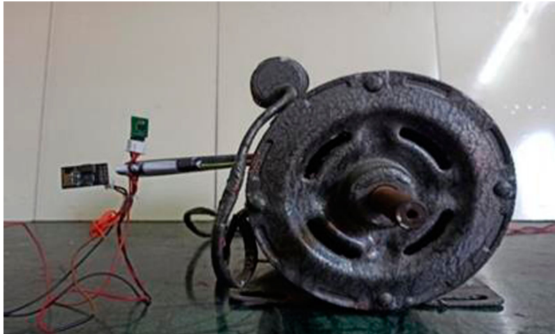
Figure 6. The hardware set-up of the proposed framework for IM rotor fault diagnosis.
