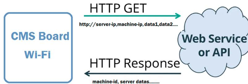
Figure 11. Block diagram of HTTP request and response.
