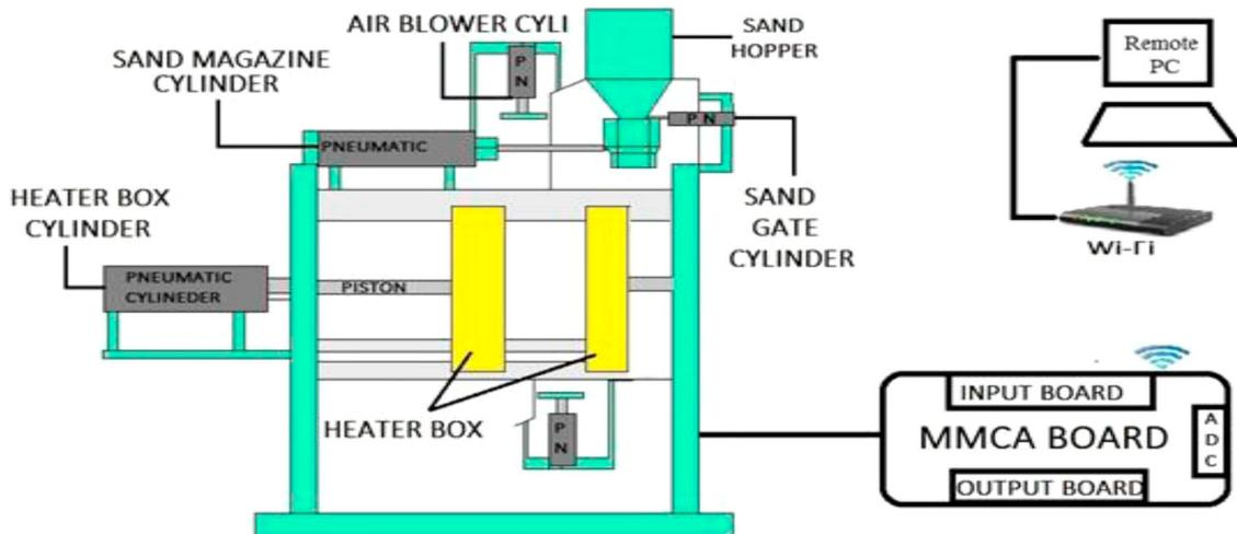
**Figure 1.** Block diagram of the CSM.
