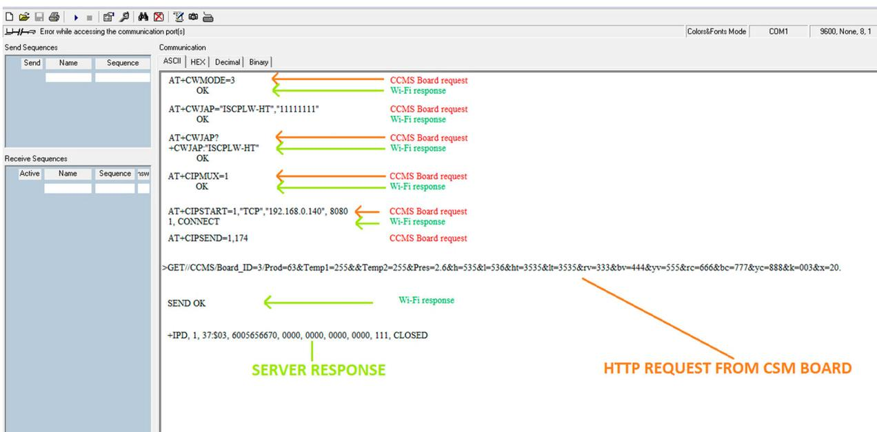
Figure 10. Esp8266 (Wi-Fi) AT commands board request and Wi-Fi response.
