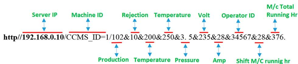
Figure 15. HTTP client request from the board to the server.
