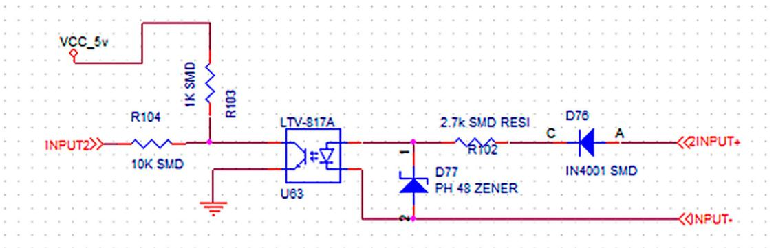
Figure 9. MMCA 24 V input circuit.
