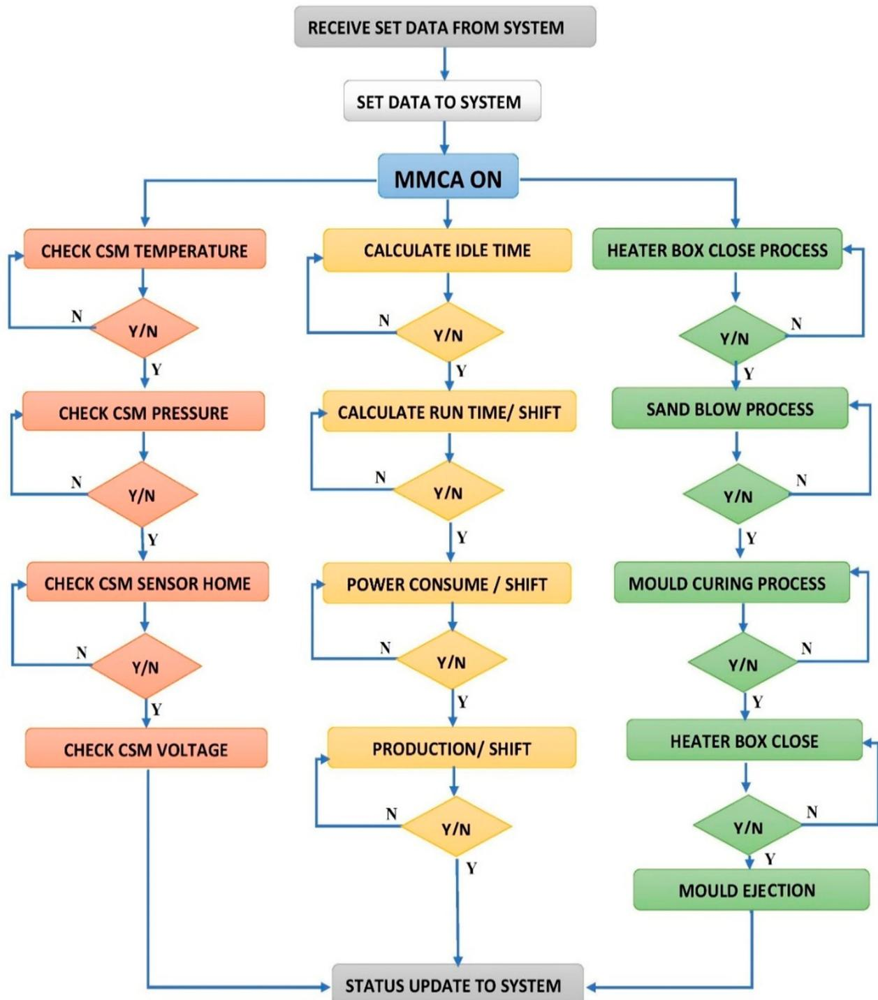
**Figure 3.** Programming logic for CSM.
