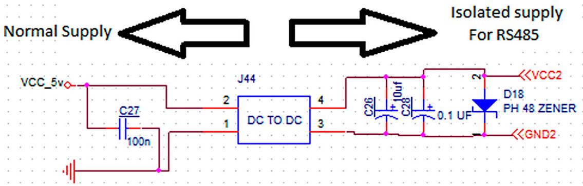
Figure 6. MMCA – RS485 DC to DC isolated power supply.
