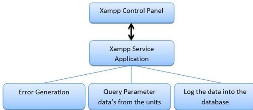
Figure 13. Architecture of system application software.
