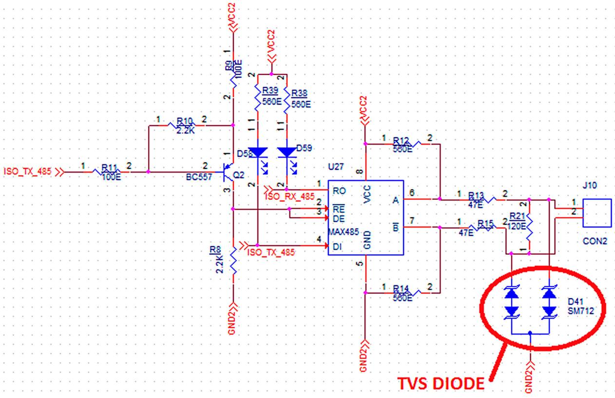
Figure 7. Isolated RS485 circuit and TVS diode.
