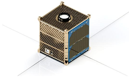
**Figure 3.** 1U CubeSat structure [27].
