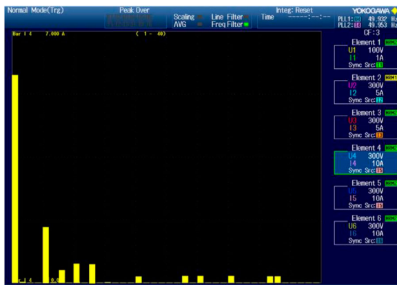
Figure 21. Experimental input current THD of 4.03%.
