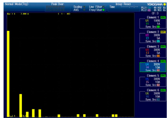
Figure 23. Experimental output voltage THD of 3.76%.
