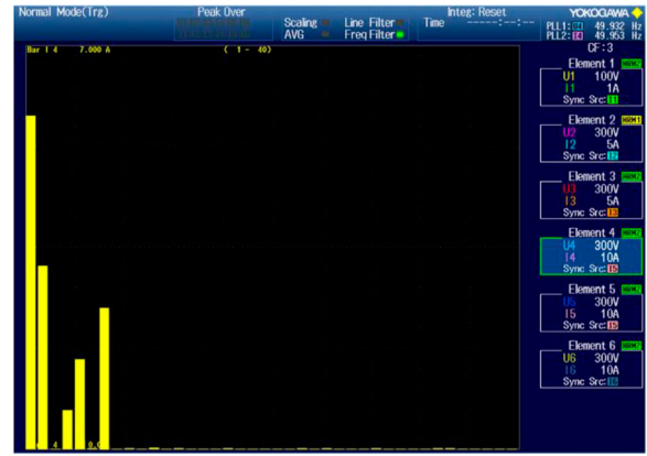
Figure 22. Experimental input voltage THD of 4.76%.
