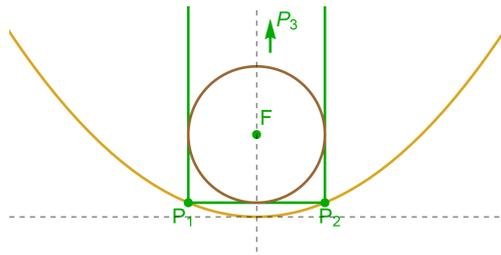
Figure 3: Construction used to derive  $r/f$  in Proposition 1. Side  $P_1P_2$  of the Poncelet triangle is perpendicular to the axis while the other two sides are parallel to it, i.e., vertex  $P_3$  lies on the line at infinity.
