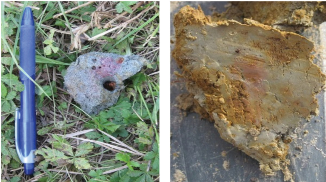
Figure 4 (Source: Vedran Rubinić). Pinkish color on the surface of a soil clod is the positive reaction after the application of the \alpha,\alpha -bipyridyl solution, proving that the soil matrix is reduced due to pronounced gleyic ( Left photograph ) or stagnic properties ( Right photograph , 8 cm wide in reality). In case no reaction to the applied solution was observed, the albic material (grey soil) would be interpreted as the iron depletion, instead as the reduced matrix.
