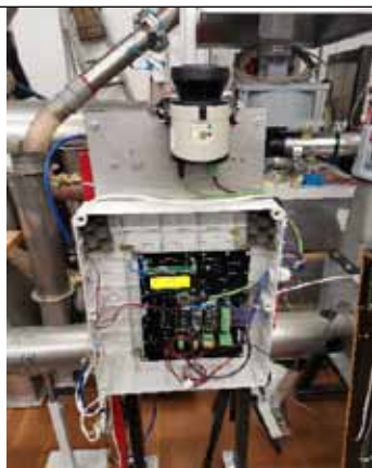
Figure 1b: Autonomous modular system for optimizing the spray mixture application process
