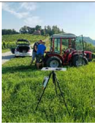
Figure 1c: Installation of DGPS measuring system close to the vineyard
