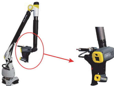
Articulated measuring arm with contact probe Model: Nikon MCAX 2.0+ Volume length accuracy: \pm 33 \mu\text{m} Point repeatability: 23 \mu\text{m}
