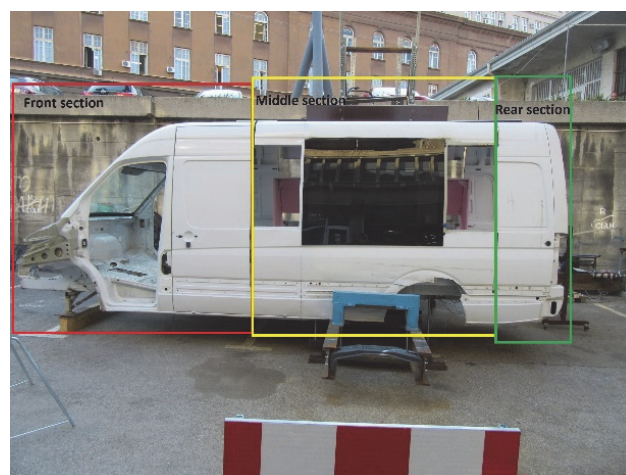
Figure 6 Body structure divided into three sections for the purpose of quasi-static loading test
